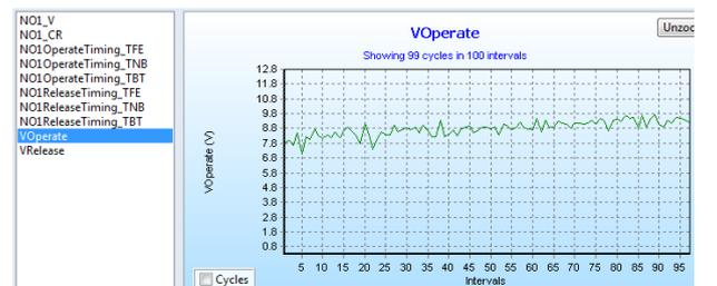
Figure 15. Operate Voltage chart by test intervals.
