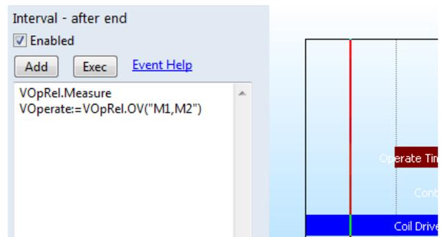
Figure 14. Programming the system to perform an Operate / Release Voltage test.
