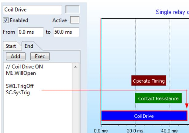
Figure .5 Actions at the end of the Coil Drive Time Slot
