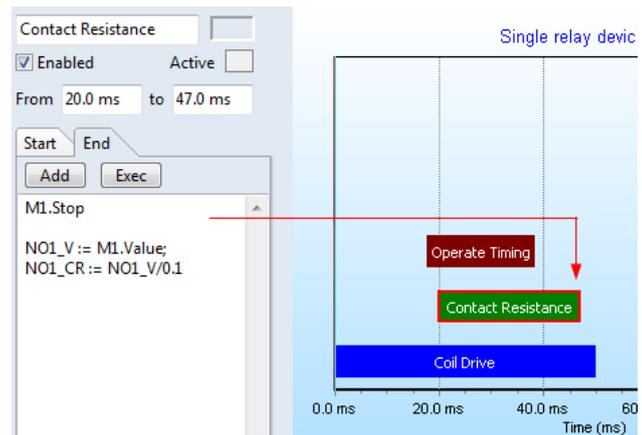
Figure 7. The Contact Resistance time slot STOP event
