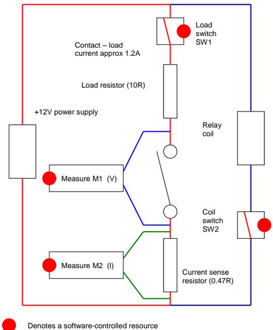
Figure 1. Simple high-power life-test circuit, e.g. automotive.
