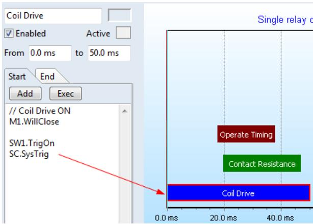
Figure 4. Actions at the start of the Coil Drive Time Slot
