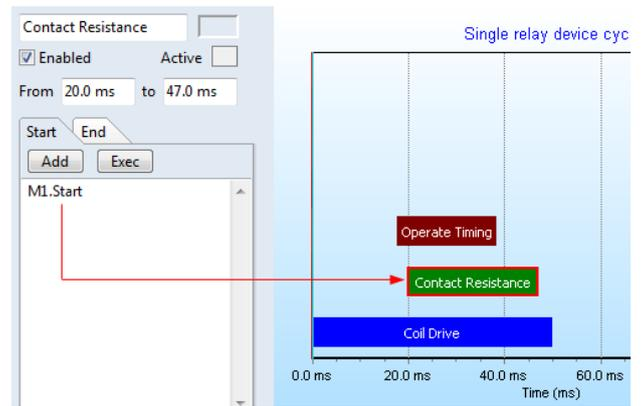
Figure 6. The Contact Resistance time slot START event
