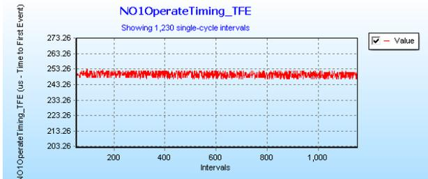
Figure 11. Operate time chart by contact cycles.
