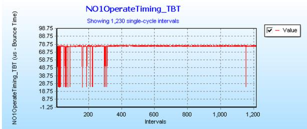
Figure 12. Bounce time chart by contact cycles.
