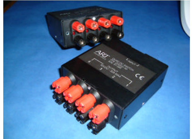
Figure 9 A typical semiconductor switch module
