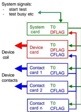
Figure 12 - Signal wiring - basic system.
