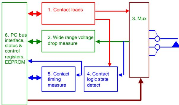
Figure 5 Contact card resources - block diagram
