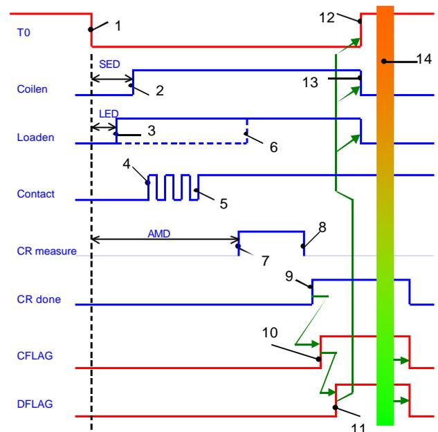
Figure 17 Example system signals – CR measurement.
