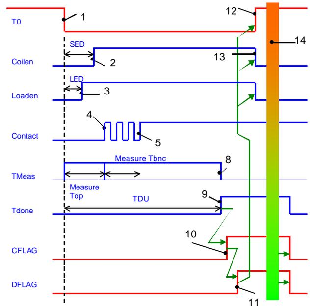
Figure 18 Example timing signals - Timing
