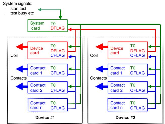
Figure 13 Signal wiring - dual system.
