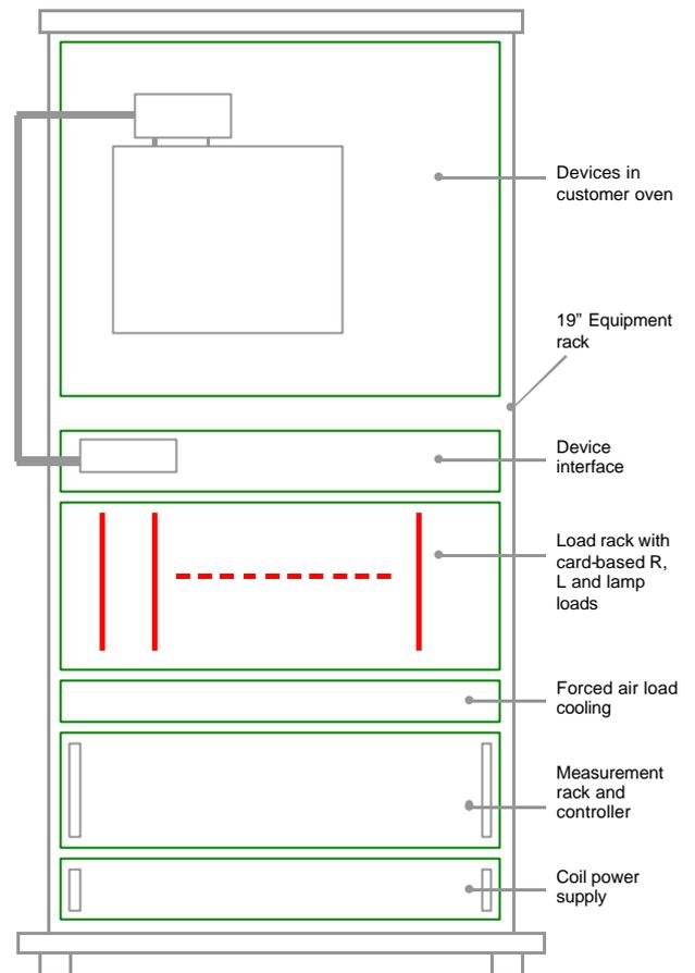
Figure 15 Rack mounted items – Reflex 50 Life Test System.
