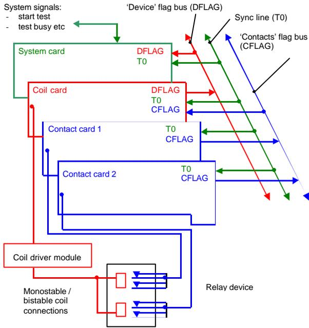
Figure 2 - Unified REFLEX architecture
