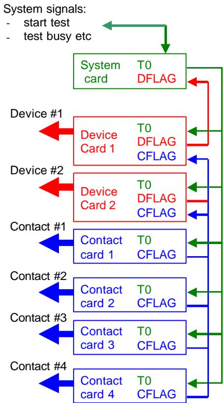
Figure 14 Life test system architecture
