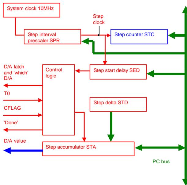
Figure 9 Block diagram, step logic
