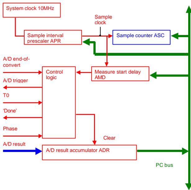
Figure 7 Block diagram, A/D integration
