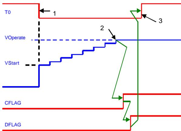
Figure 10 - Operate Voltage measurement
