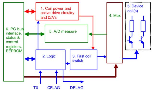
Figure 8 - Device card resource block diagram
