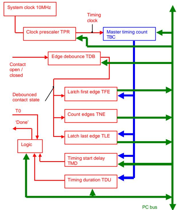
Figure 6 Block diagram, timing measurement
