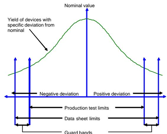
Figure 5 A typical result distribution for a test parameter
