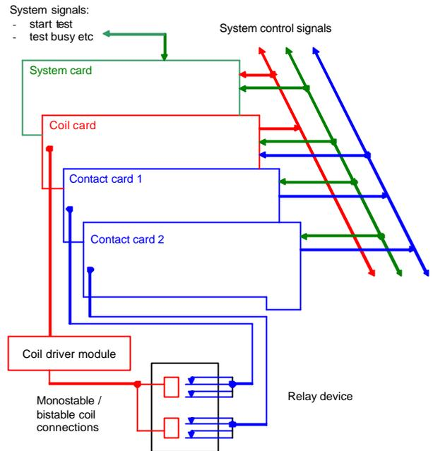
Figure 1 A parallel architecture test system
