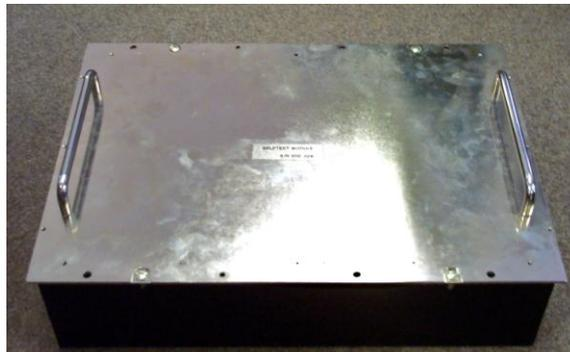
Figure 7 - Fixture adapter for device under test, top view.
