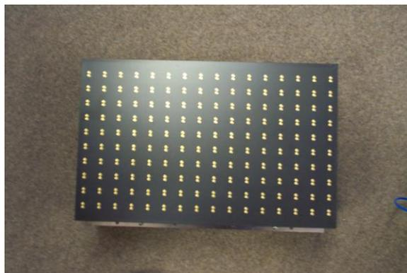
Figure 8 - Fixture adapter bottom view shows Kelvin connections
