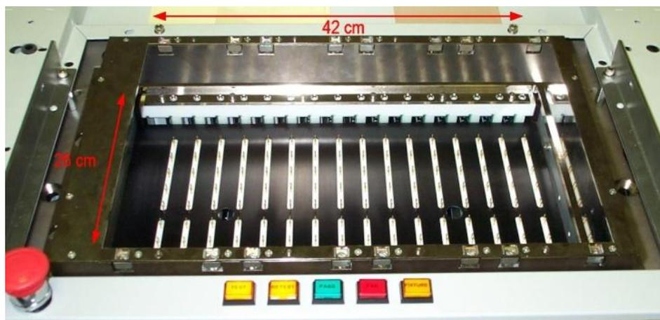
Figure 9 - The 'bed of nails' that connect to the fixture adapters.
