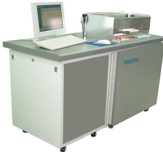
Figure 5 - The Reflex 950 Passive Component Tester.
