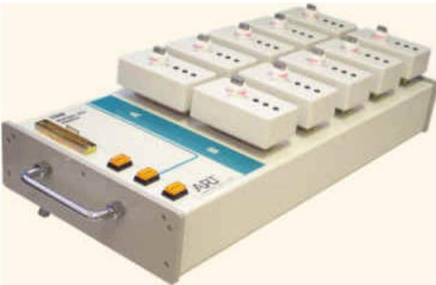
Figure 9 A multi-way test fixture which can speed operator-based test.
