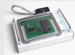
A semi-automated calibration/self-test module ASY0270
